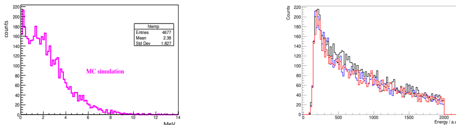
Figure 3. Energy release: Monte Carlo simulation and experimental data for 51 MeV-photon irradiation of SpaCal. The different colours of line correspond to a few small falling angles of a photon beam (the right panel)
