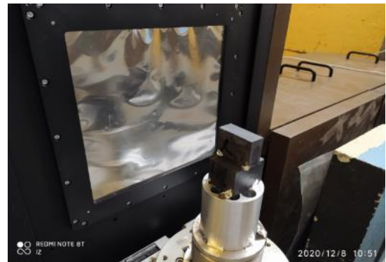
Figure 2. The heterogenous quartzite rock sample on top of the turntable.
