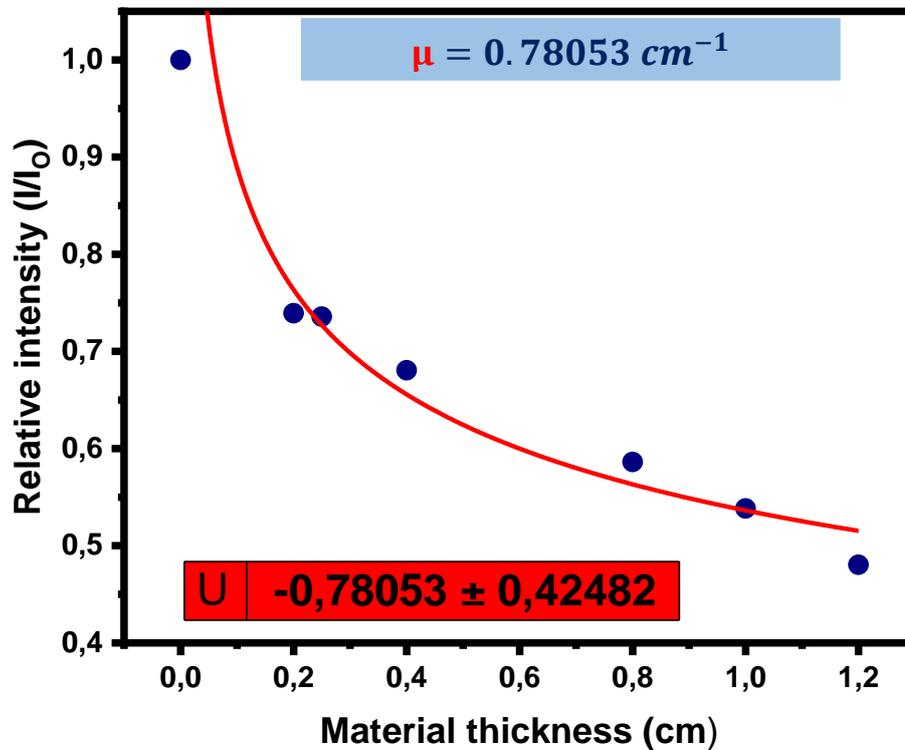
Figure 9: Attenuation of Cs-137 radiation through Copper shielding.
