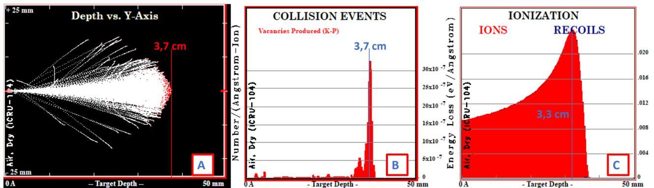
Figure 11: STIM simulating the propagation of Alpha particles in the air
