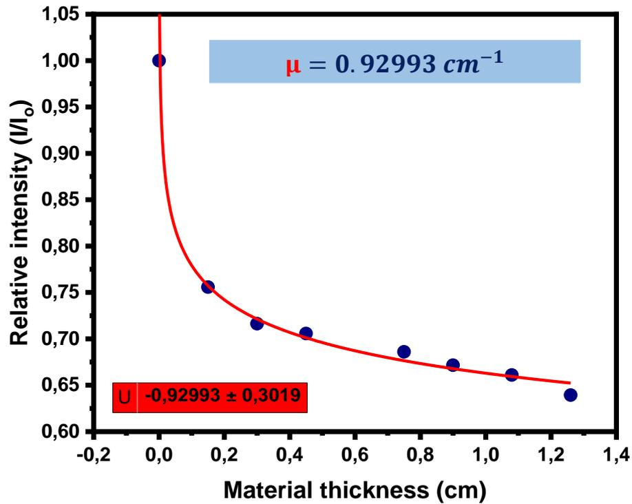
Figure 8: Attenuation of Cs-137 radiation through Aluminium shielding.
