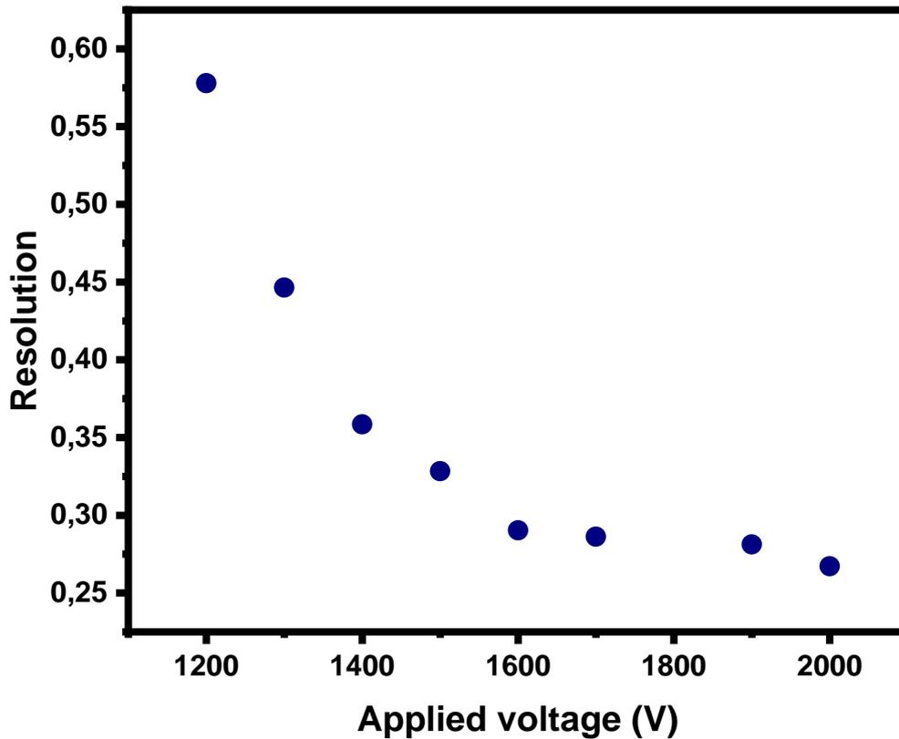
Figure 4: Showing the resolution curve of a BGO detector given as a function of Applied Voltage V.
