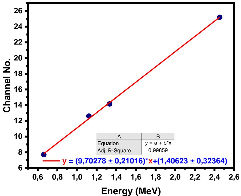
Figure 7: Calibration curve for NaI detector.
