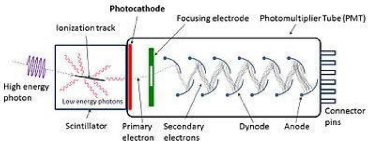
Figure 2: Schematic diagram of a scintillator detector fitted with a photomultiplier tube (PMT).
