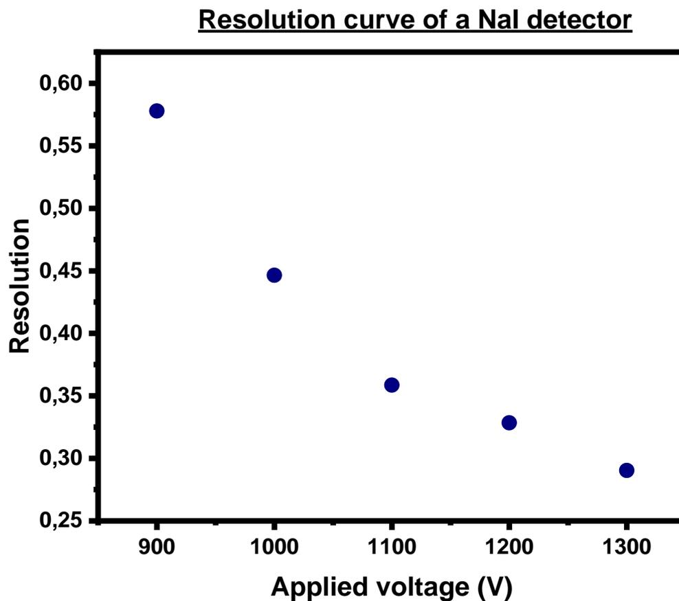
Figure 6: Showing the resolution curve of a NaI detector given as a function of Applied Voltage V.
