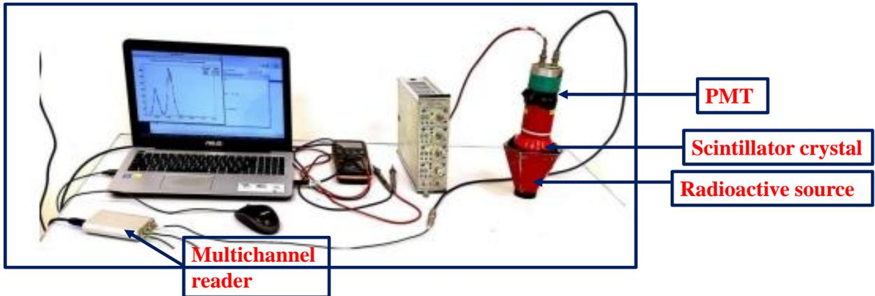
Figure 3: Scintillation detector measurement setup.
