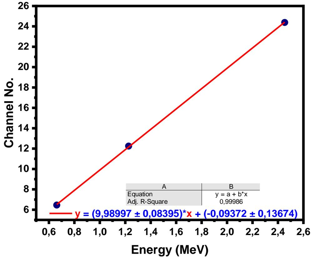
Figure 5: Calibration of BGO detector.
