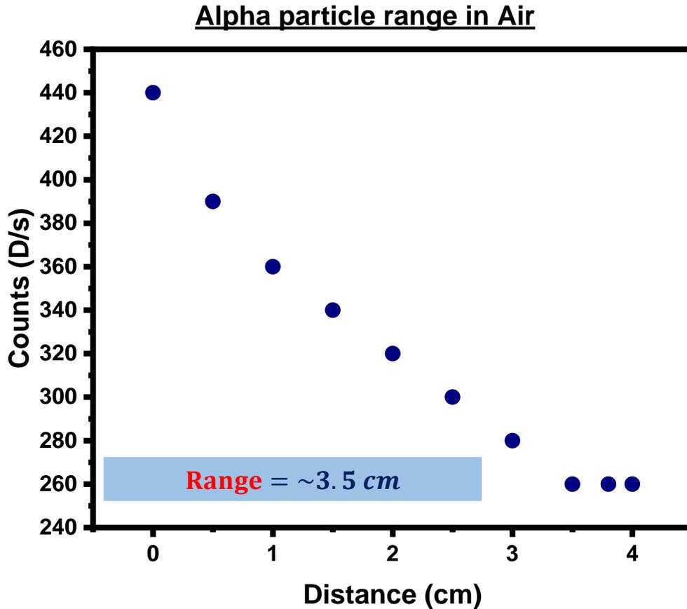
Figure 10: Alpha radiation counts observed by a plastic detector
