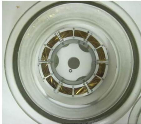
Fig.2: **a)**. Schematic overview of Target assembly with the hot catcher: 1 - split collimator; 2 - beam flux measuring foil; 3 - target; 4 - separating foil; 5 - graphite foil; 6 - heater. **b)**. The photo of the rotating target cassette in assembly. 6 packs, 2 windows at 14mm width each. Target material  $^{242}\text{Pu}$  in oxide state put on the Ti 2  $\mu\text{m}$  thick foil .
