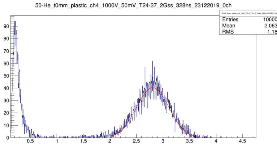
Figure 14 Energy spectrum of alpha at distance = 0 cm from the plastic detector
