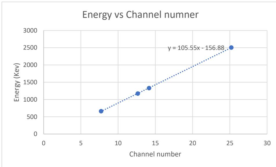
Figure 10. Calibration curve for NaI detector
