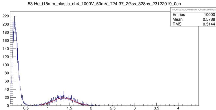
Figure 15. Energy spectrum of alpha at distance = 1.5 cm from the plastic detector
