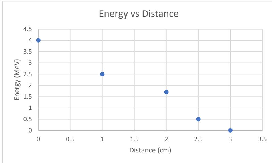
Figure 23. Energy of alpha with distance from the pexel detectors
