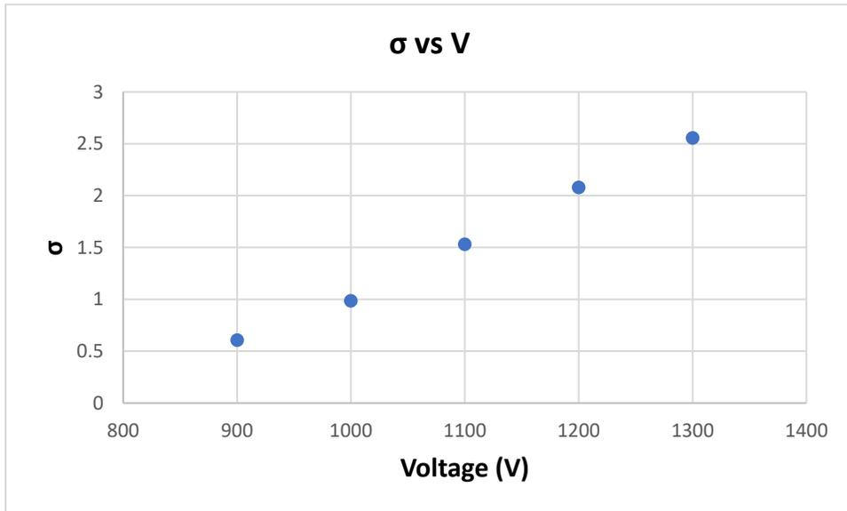
Figure 8. Relationship between the signal and applied voltage
