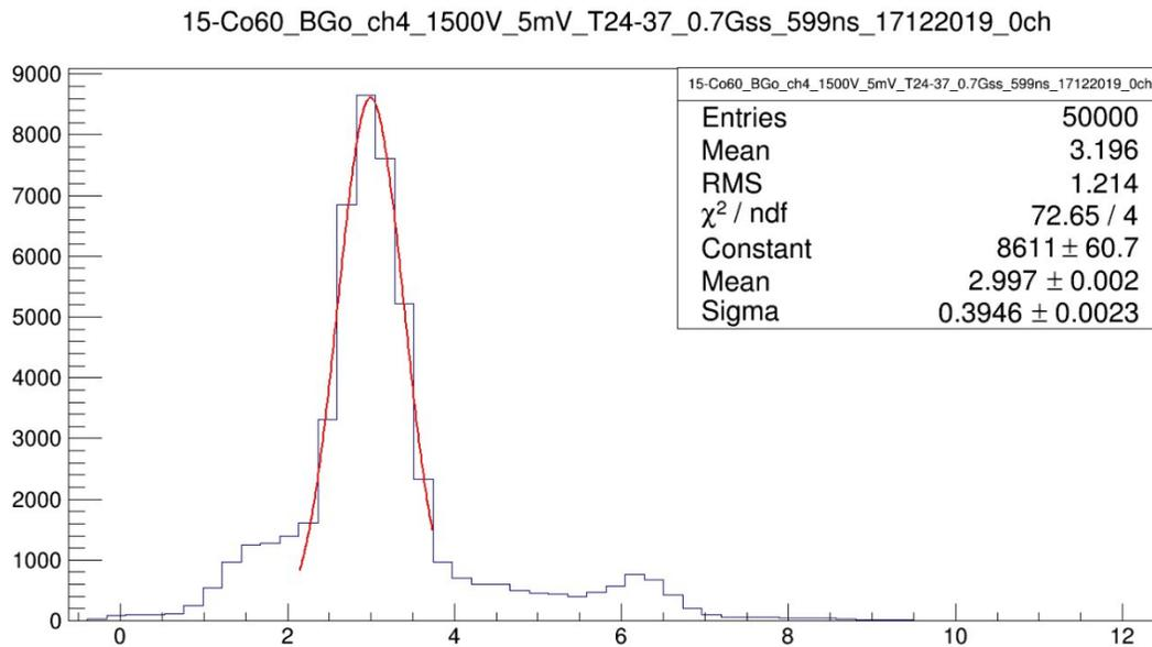
Figure 2. Spectrum of Co60 using BGO detector at 1500 applied voltage.
