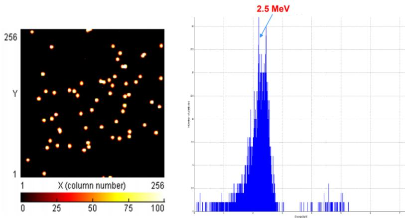
Figure19. Alpha spectrum at 1 cm
