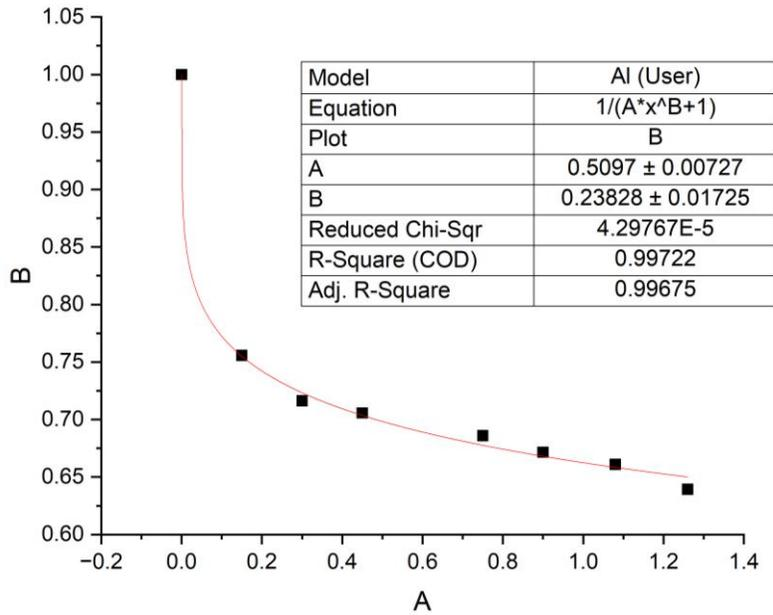
Figure 12. Attenuation of gamma by Al
