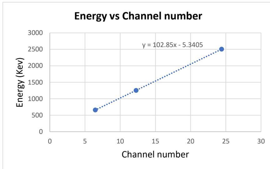
Figure 6. Calibration curve of BGO detector
