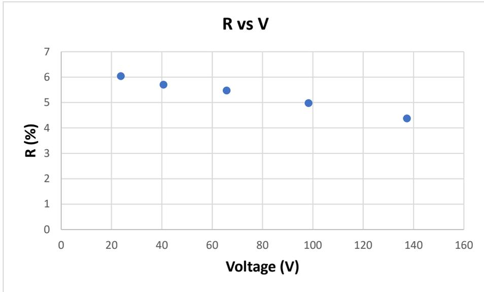
Figure 7. Relationship between the resolution and applied voltage
