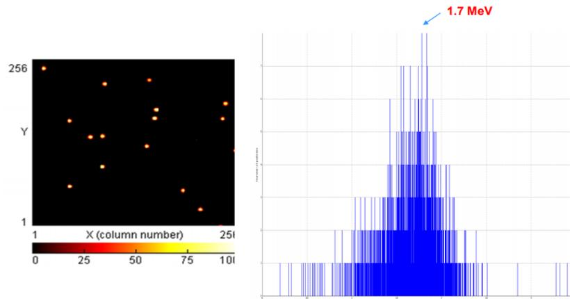
Figure 20. Alpha spectrum at 2 cm
