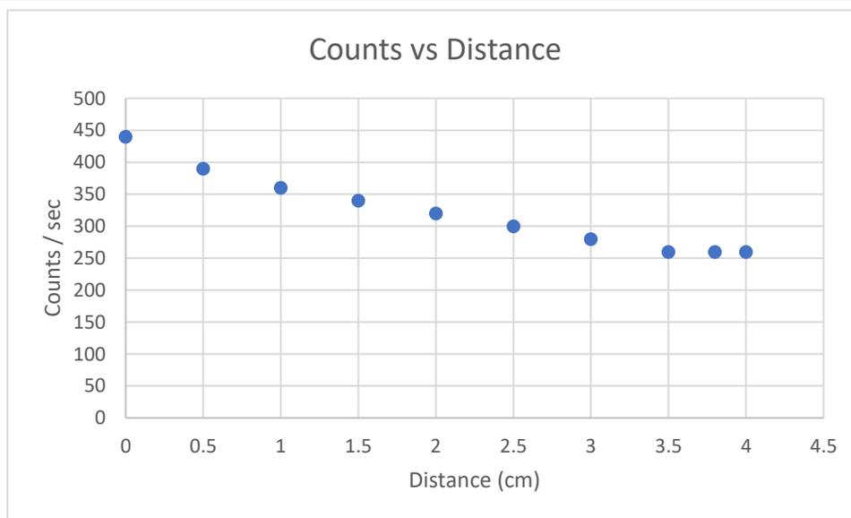
Figure 17. Number of counts per second with the distance from the plastic detector
