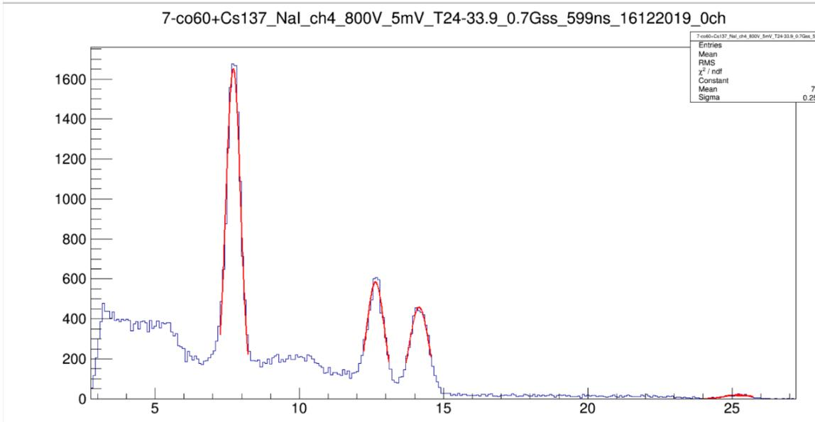
Figure 9. Signal of known sources (Cs137 + Co60) taken by NaI detector
