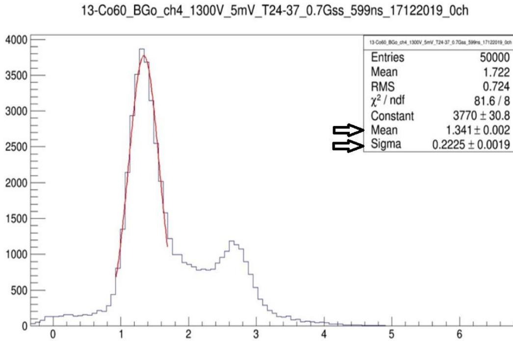
Figure 1. Spectrum of Co60 using BGO detector at 1300 applied voltage.
