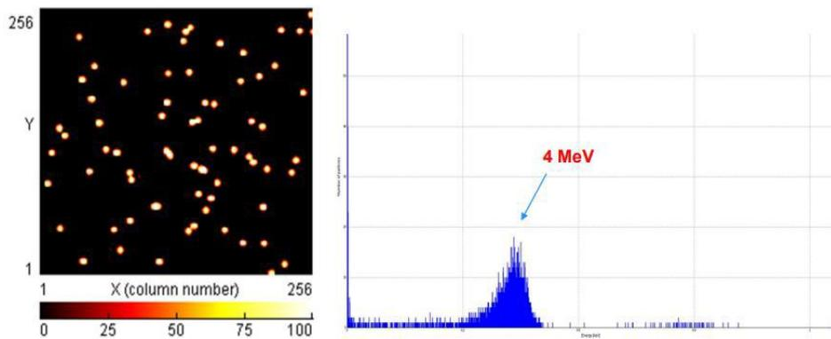
Figure 18. Alpha spectrum at 0 cm
