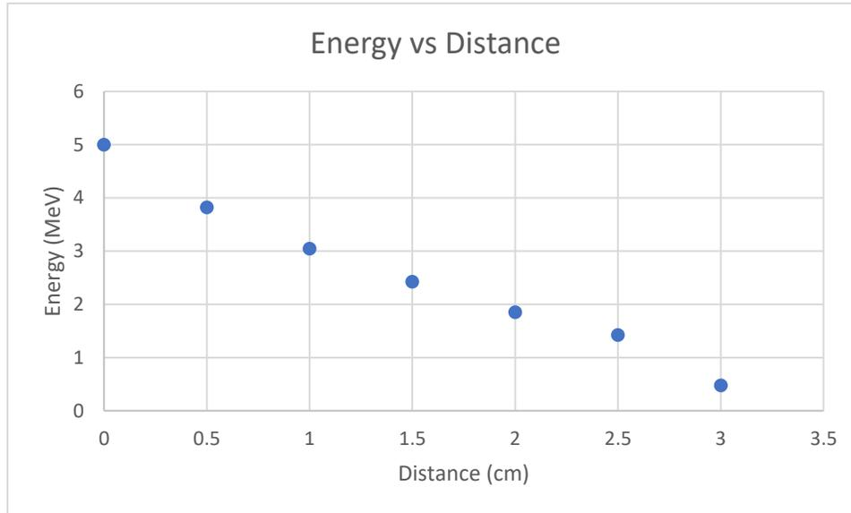
Figure 16. Energy of alpha in air with distance from the plastic detector
