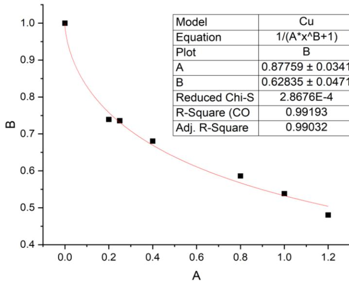
Figure 13. Attenuation of gamma by Cu
