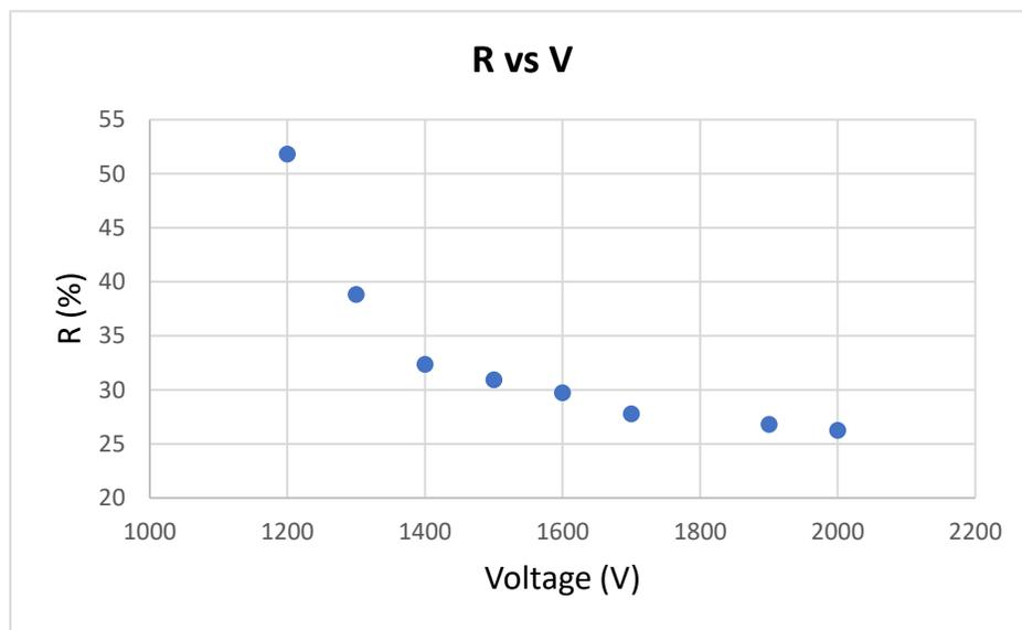
Figure 3. Relationship between the resolution and applied voltage
