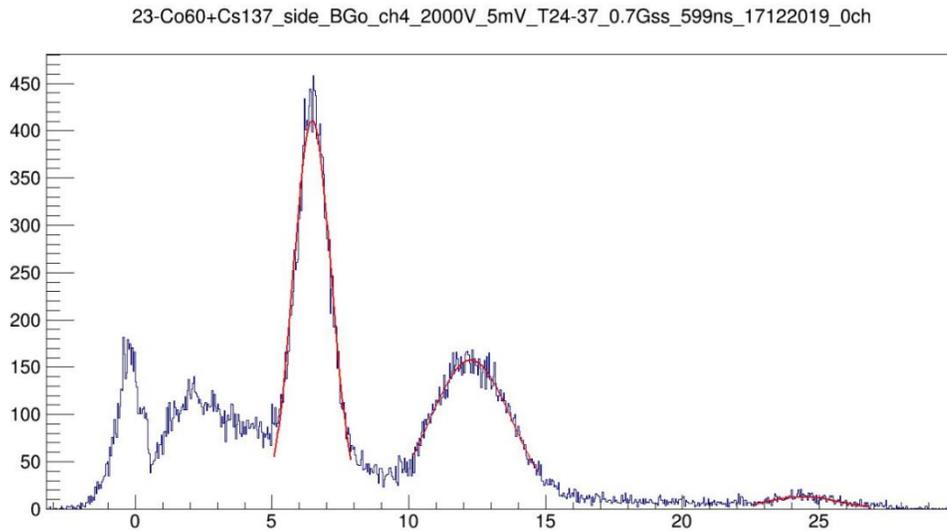
Figure 5. Signal of known sources (Cs137 + Co60) taken by BGO detector
