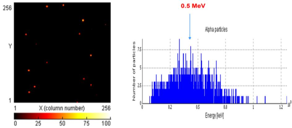
Figure 21. Alpha spectrum at 2.5 cm
