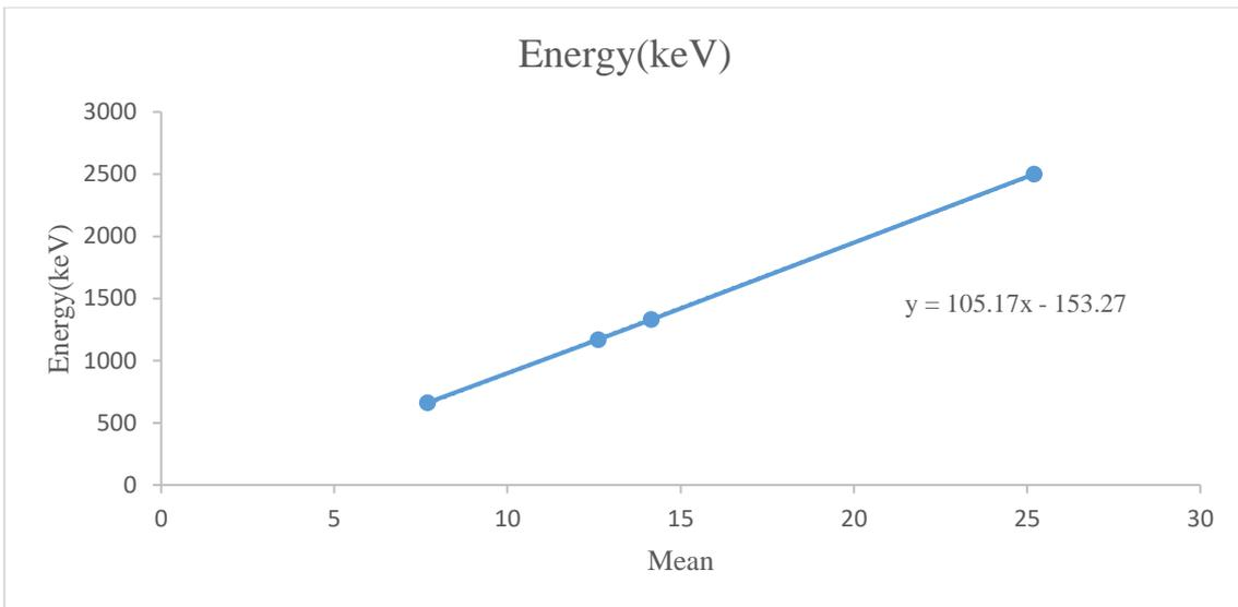
Figure 19, Energy calibration function for Cs-137 and Co-60 spectrum from NaI detector measurements.
