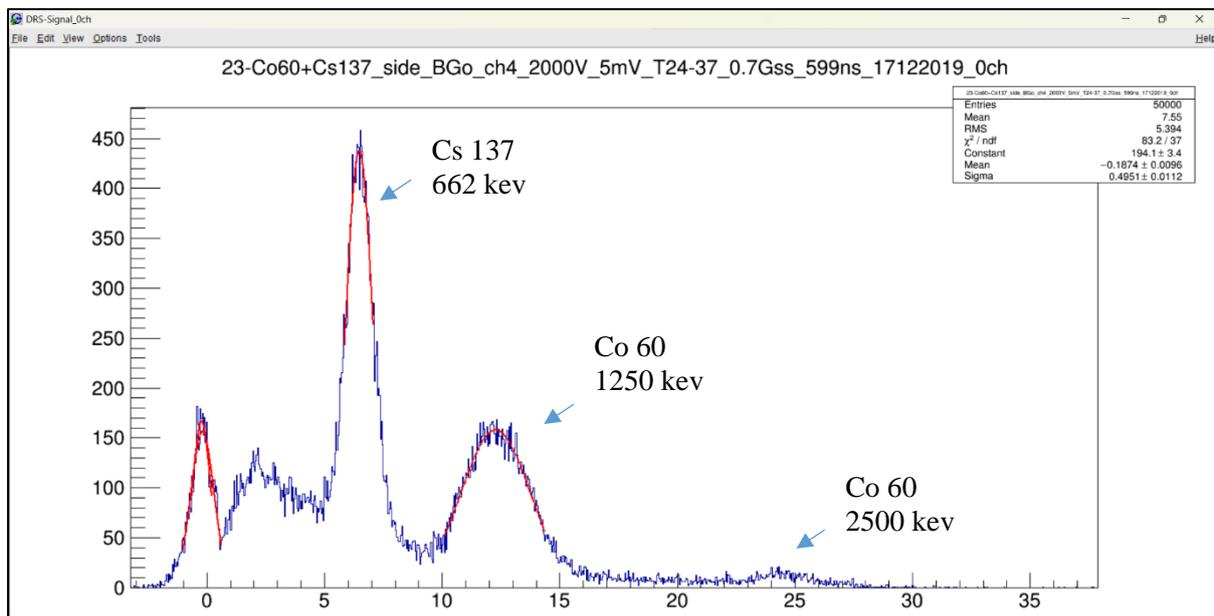
Figure 10 The energy spectrum of Cs-137 and Co-60 from BGO detector measurements at 2000V.
