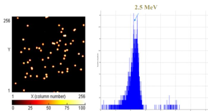
figure 31, Absorption of  $\alpha$ particle energy at 1 cm in the air
