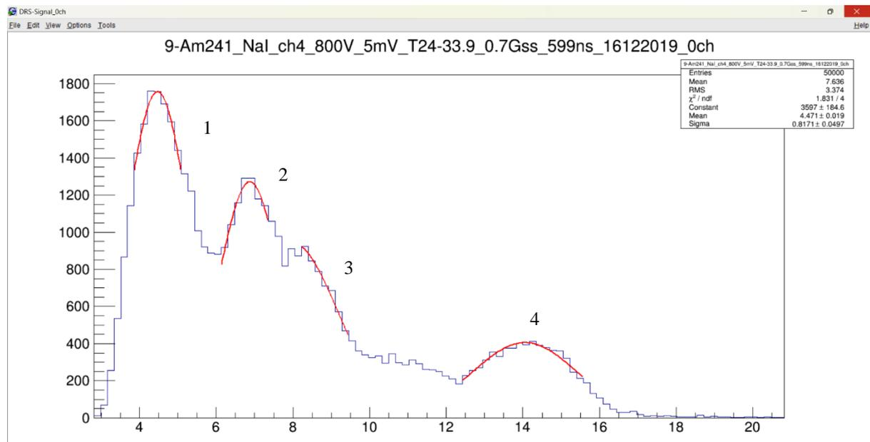
Figure 19, The energy spectrum Unknown source NaI detector measurements at 800V
