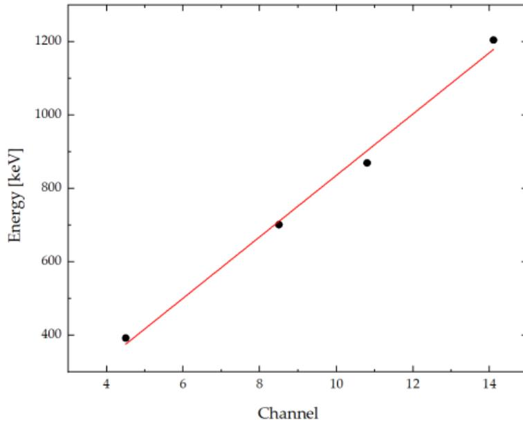
Figure 20, Energy calibration Unknown source NaI detector measurements
