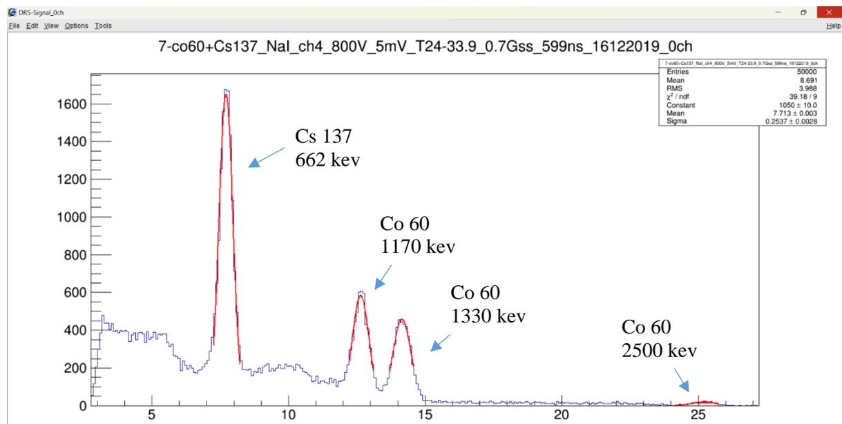
Figure 18, The energy spectrum of Cs-137 and Co-60 from NaI detector measurements at 800V.
