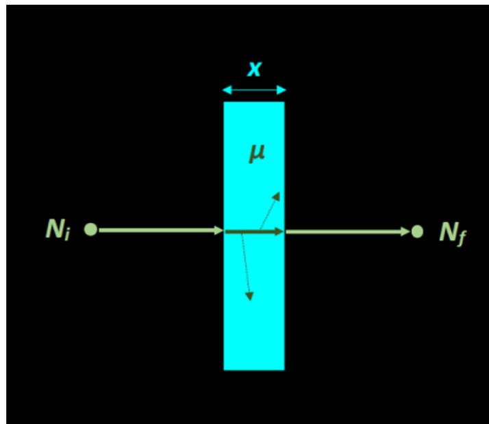
Figure 25, Energy Attenuation of  $\gamma$  radiation coefficient
