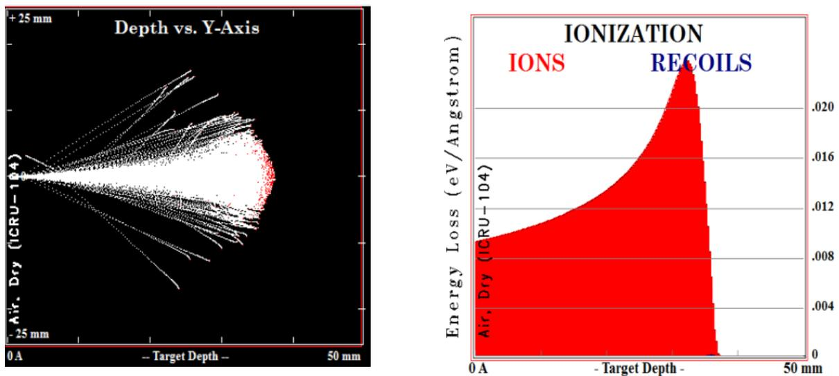
Figure24, Depth and Bragg curve of alpha particles in 5 cm air.
