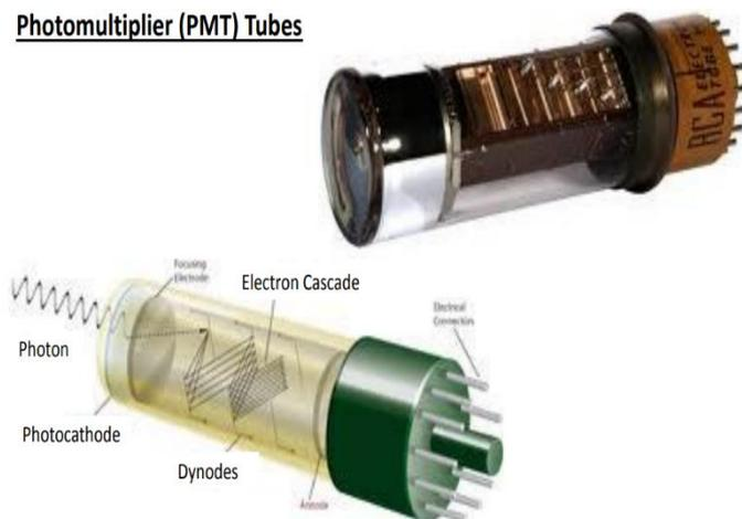
Photomultiplier tubes are commonly used as photodetectors in scintillator detectors. They consist of a photocathode and a series of dynodes. When the scintillation light strikes the photocathode, photoelectrons are emitted and focused onto the first dynode. This process triggers a cascade of electron multiplication, as
