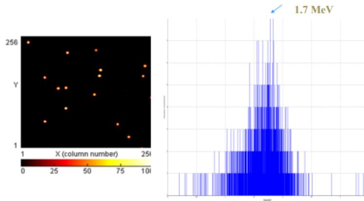
Figure 32, Absorption of  $\alpha$ particle energy at 2 cm in the air
