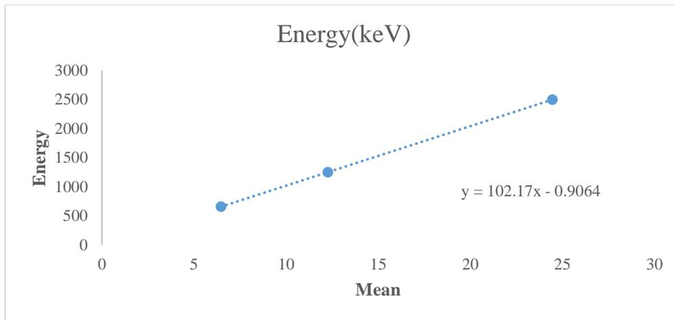
Figure 11, Energy calibration function for Cs-137 and Co-60 spectrum from BGO detector measurements.
