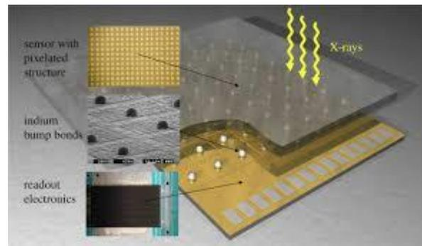
Figure 28 Pixel detectors
