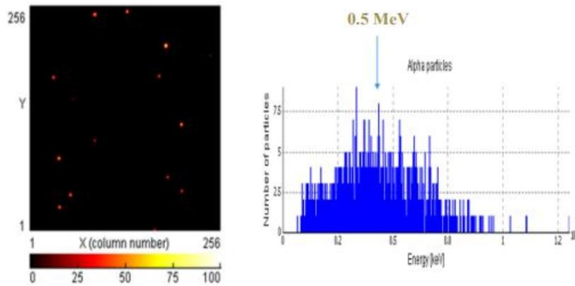
figure 33, Absorption of  $\alpha$ particle energy at 2.5 cm in the air
