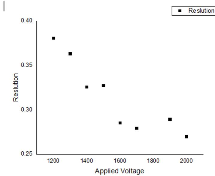
Figure 9, The relation between resolution and applied voltage for BGO detector. Resolution improves with increasing voltage.
