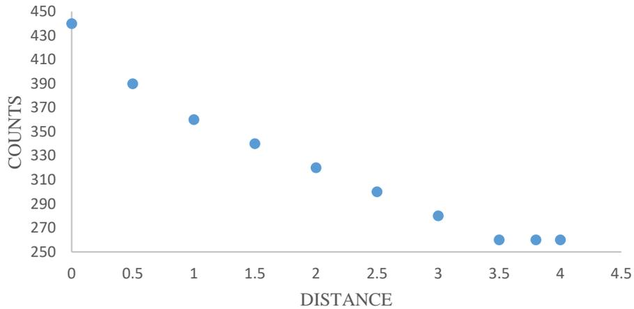
Figure23, Alpha radiation counts observed by a plastic detector.
