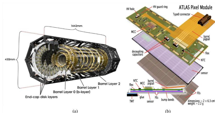
Figure 29 Pixel detectors
