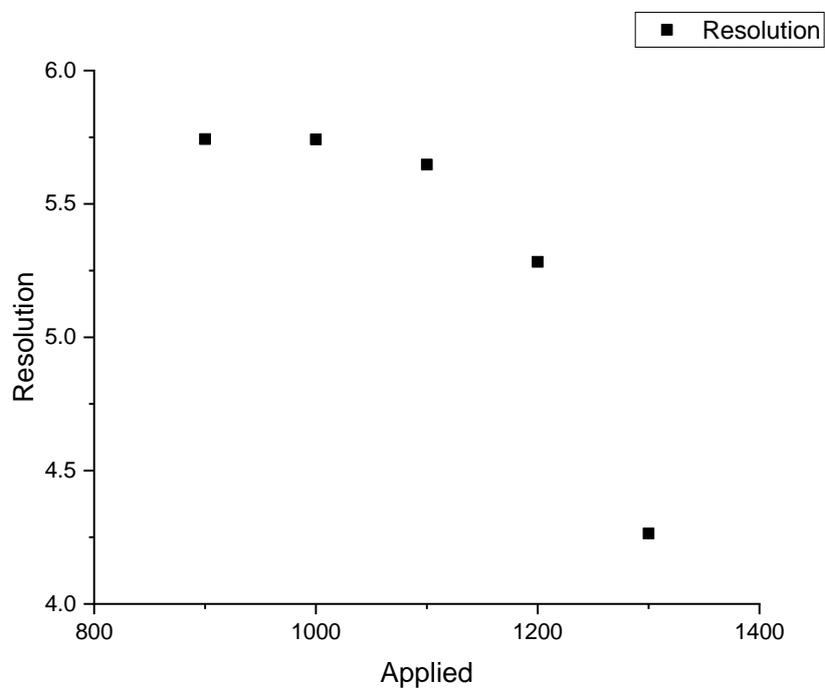
Figure 17, The relation between resolution and applied voltage for NAI detector. Resolution improves with increasing voltage.
