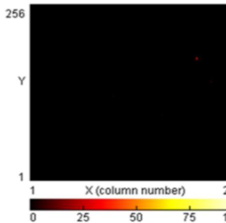
Figure34, No  $\alpha$ -particles are detected which means maximum of  $\alpha$ -particle range is 3 cm in this case.
