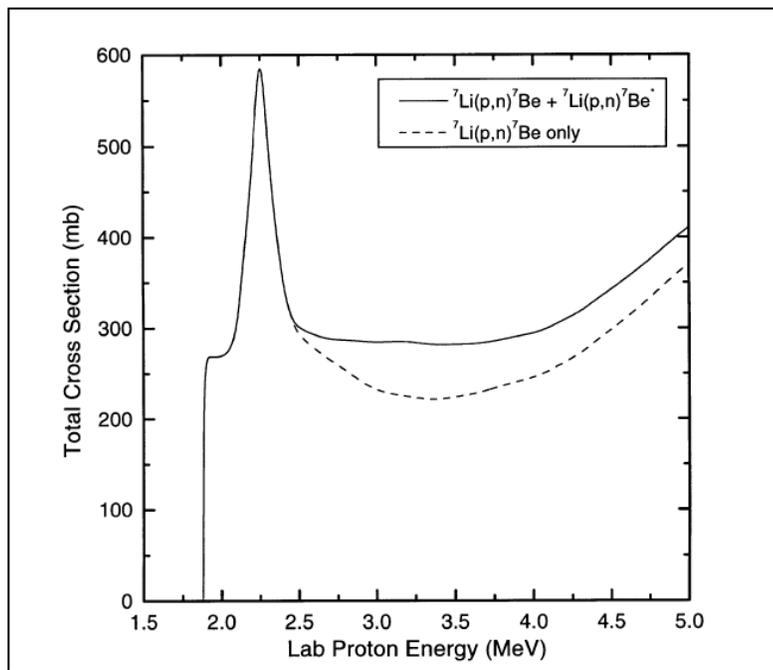
Figure 2: Total (p,n) Cross Section for  ${}^7\text{Li}$ . (H. Liskien and A. Paulsen 1975)
