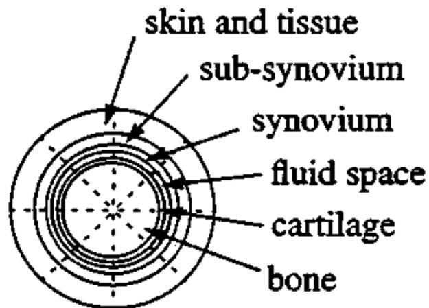
Figure 4: Knee phantom schematic
