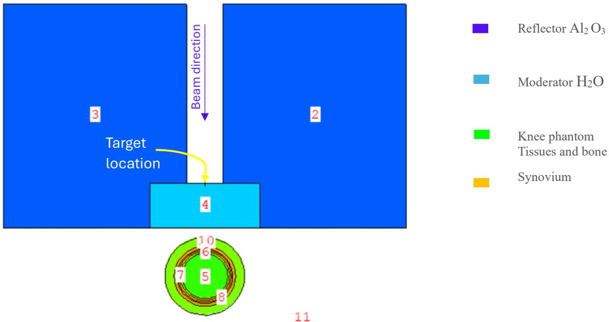
Figure 3: Geometry of MCNP model used for BNCS feasibility study
