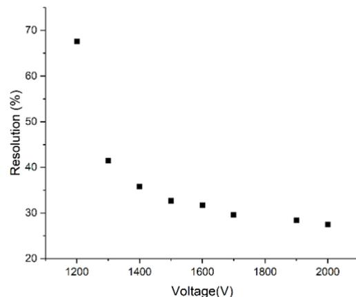
As the voltage increased, the resolution percentage decreased. This means the detector gave clearer and more accurate results at higher voltages. The peaks in the spectra became sharper, which helps in better identifying the energies.
