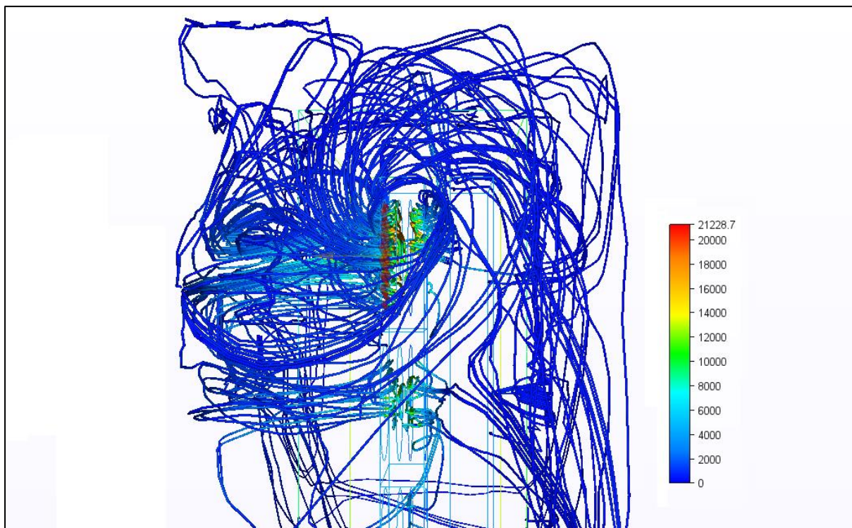
Fig. 18: Visualisation of the Movement of Air (Scale is Velocity Magnitude in cm/s) as forced by the Fans within the Rack Volume at 5000RPM.
