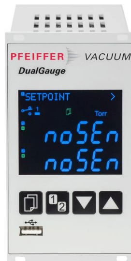
Figure 8. The PFEIFFER gauge controller used in PPACs' setup.
