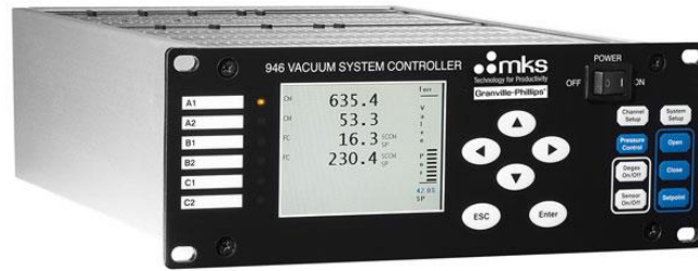
Figure 9. The MKS vacuum system controller used in PPACs' setup.
