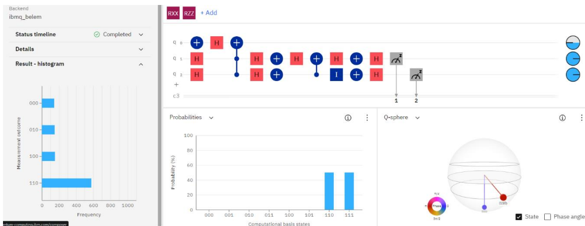
Figure 14.- Grover algorithm circuit results for finding the state |1,1\rangle . At the left is the histogram obtained by the ibmq_belem quantum computing after performed the algorithm.
