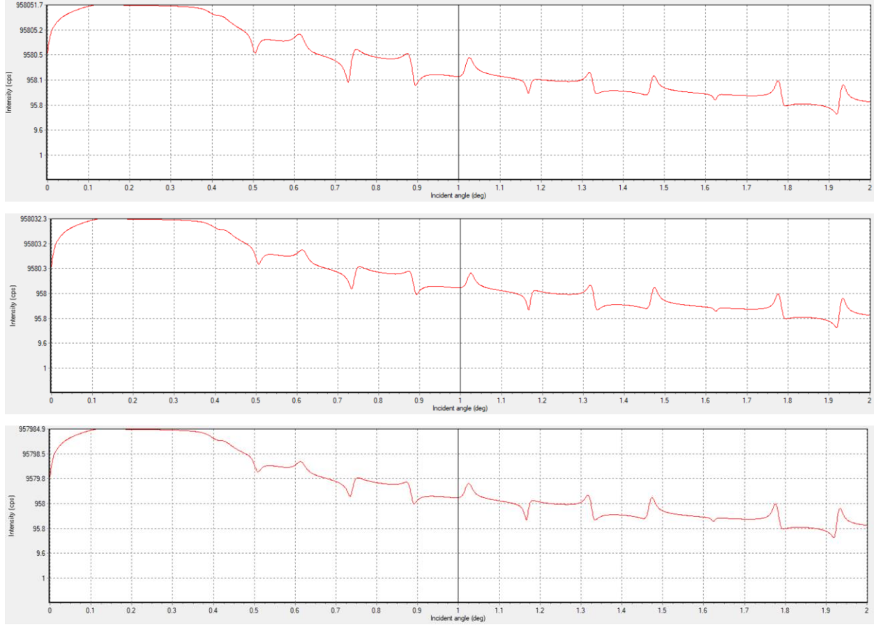
Figure 25. X-ray reflectivities for investigated heterostructures with the roughness of Gd layer of 0, 1, 2, and 3 nm, from top to bottom.
